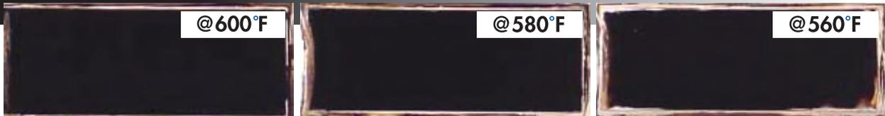
The Panel Coker test is above and beyond the NMMA's TC-W3® testing. Cleaner panels represent a cleaner burning oil with less impurities that will result in less engine deposits and reduced exhaust smoke.
